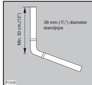
When discharging into a standpipe ensure that the top of the curve in the hose end is no more than 90cm (35.4") and no less than 60cm (23.6") above floor level. The upright standpipe should have a minimum length of 30cm (12") from the bottom of the elbow to the top of the pipe (see diagram). Make sure that it is designed in such a way, that the end of the drain hose cannot be covered with water.
