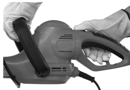
Figure 3-8: Releasing trigger switch to stop trimmer
