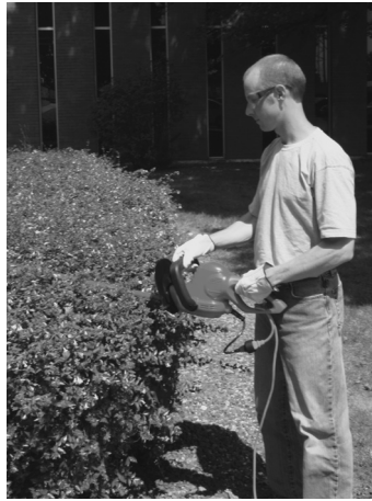
Figure 3-13: Proper clothing, stance, grip, and extension cord maintenance
