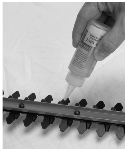
Figure 4-3: Oiling cutter blades
