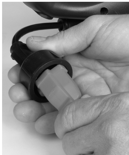
Figure 3-1: Plugging trimmer power cord into extension cord
