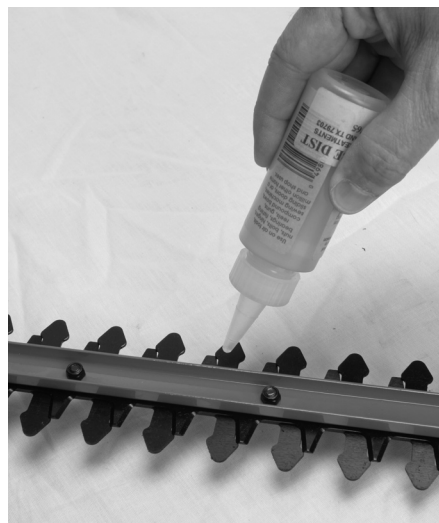
Figure 4-3 : Lubrification des lames
