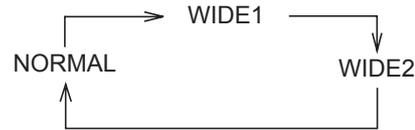
Release the "DISPLAY MODE" button; 6 seconds later, a full screen will be displayed in the selected mode.
