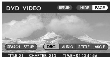
Highlight the “DRC” switch on the screen with the remote control joystick, then press the “ENTER” button. The display will switch to the dynamic range control selection screen.
