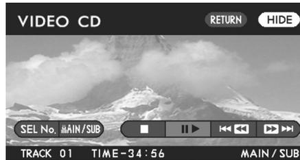
To make the switches disappear from the screen, push the remote control’s “CURSOR” button again or highlight the “HIDE” switch on the screen with the joystick and then press the “ENTER” button. If you highlight and execute the “HIDE” switch, the TRACK number and playback time at the bottom of the screen also disappear.
