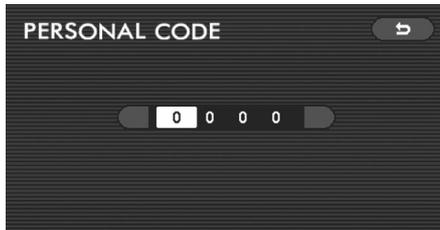
With a DVD video disc loaded in the player, access the SETUP MENU screen. Highlight the “PARENTAL LOCK” with the remote control joystick, then press the “ENTER” button. The display will change to the “PERSONAL CODE” screen.
