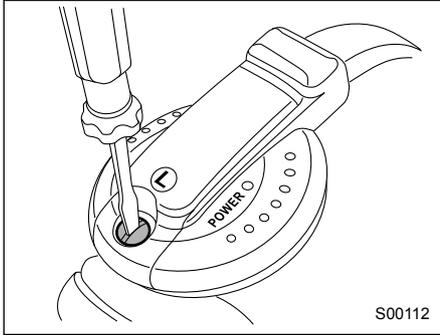
Remove the battery cover on the left earpiece by loosening the screw with a flat-head screwdriver.
