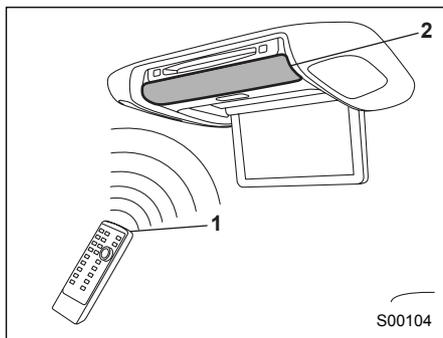
To use the remote control, direct its signal-emitting eye toward the signal reception window of the display.
