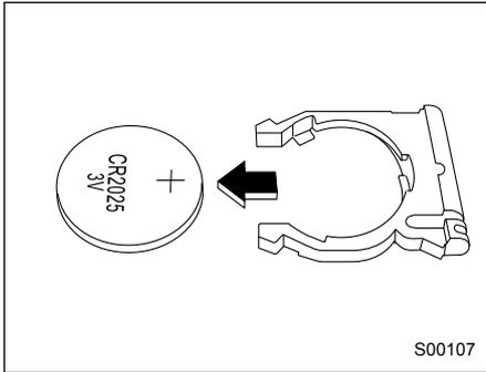
Install a new battery (Type CR2025 or equivalent) in the holder. Make sure the battery's positive (+) side and the "+" mark on the holder are on the same side. Slide the battery holder into the remote control until it clicks.
