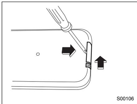
While holding the battery holder pushed in the direction of the arrow with your fingernail inserted in the slot, slide out the holder in the direction of the arrow using a cross-head mini screwdriver.
