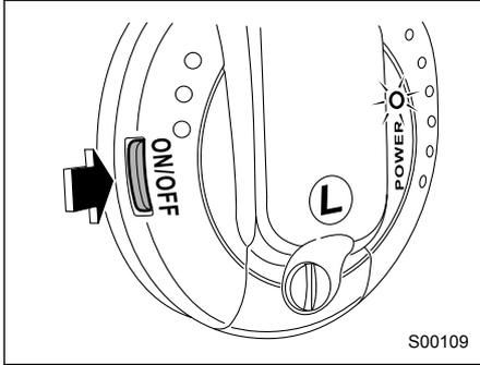
Press the ON/OFF button on the left earpiece to turn on the headphones: the POWER lamp will come on.
