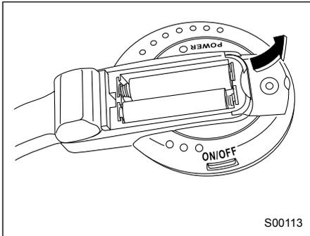
Remove the old batteries and install new ones (two AAA batteries). Pay careful attention to the (+) and (-) marks on the battery case. Reinstall the cover in position by tightening the screw with a flat-head screwdriver.
