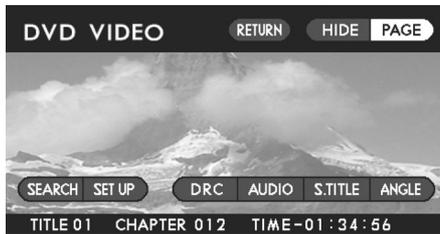
When playing a DVD video disc, different control switches are displayed on the screens for Menu 1 and Menu 2 (Menu 1 screen appears first when the “CURSOR” button is pressed). Switch between the two screens when necessary by highlighting the “PAGE” switch on the screen with the joystick and then pressing the “ENTER” button.
