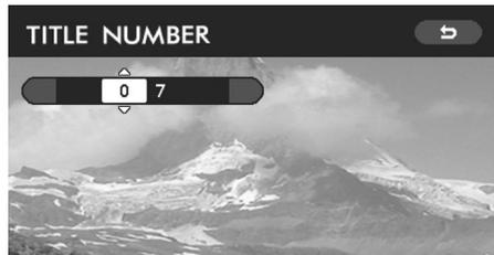
Enter the title number using the remote control joystick, then press the "ENTER" button. The player will play back the disc beginning with the specified title. To revert to the original video screen, highlight the "5" switch with the joystick, and then press the "ENTER" button.
