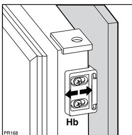
10. Place the small square on the guide again and fix it with the screws supplied.
