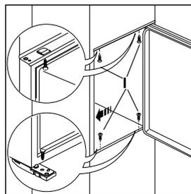
3. Open the door and push the appliance against the side of kitchen furniture opposite to that of the appliance hinges. Fasten the appliance with 4 screws (I) provided in the kit included with the appliance.
