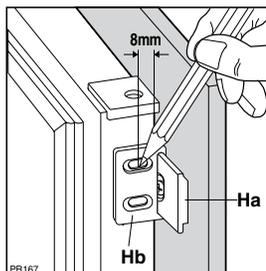
8. Open the appliance door and the furniture door at 90°. Insert the small square (Hb) into guide (Ha). Put together the appliance door and the furniture door and mark the holes as indicated in the figure.
