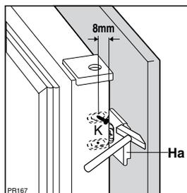
9. Remove the squares and mark a distance of 8 mm from the outer edge of the door where the nail must be fitted (K).
