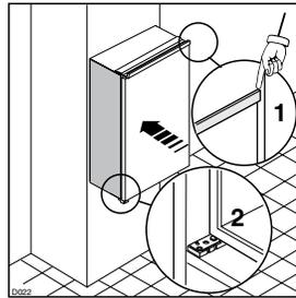
1. Fit the appliance in the niche by making sure that it stands against the interior surface of the unit on the side where the door hinges of the appliances are fitted. Insert the appliance until the upper strip butts up against the unit (1) and make sure that the lower hinge is in line with the surface of the unit (2).
