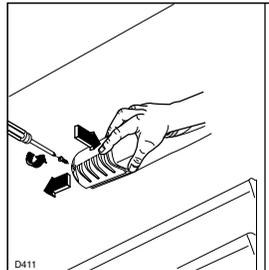
2. Unscrew the bulb and replace it with a new 15 watt bulb (available from your nearest Service Force Centre).
