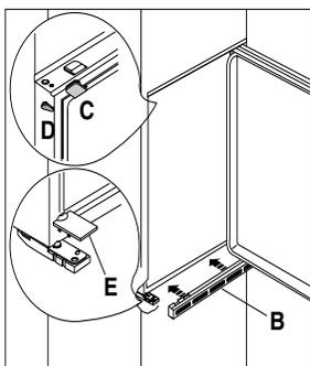
4. Snap vent grill (B) and hinge cover (E) into position.
