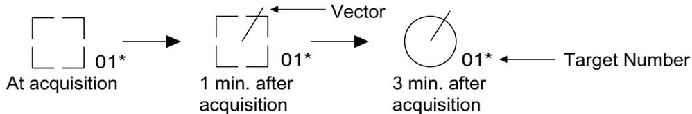
\* = Target number shown when TARGET ID NUMBER is turned on in the ARP SETUP menu.
