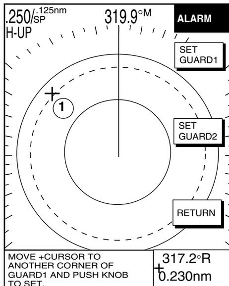
(1) Drag cursor to top (or bottom) corner for guard zone and press the SET GUARD1 or SET GUARD2 soft key.
