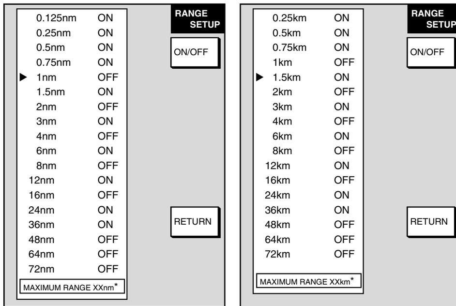
\* = Max. range depends on network radar used and is set on the network radar at installation.
