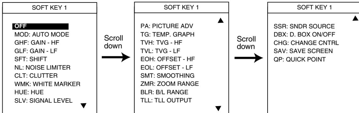
5. Select function desired with the **Cursor pad**, then press the **ENTER** soft key or **ENTER** knob to register your selection.
