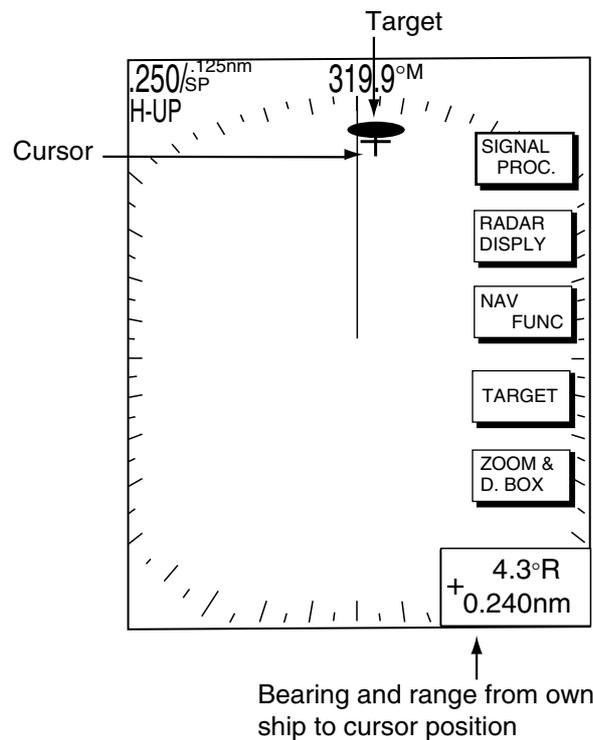
*How to measure range to a target with the cursor*
