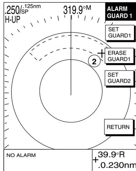
(2) Drag cursor diagonally to bottom (or top) corner for guard zone and press the [ENTER] knob.
