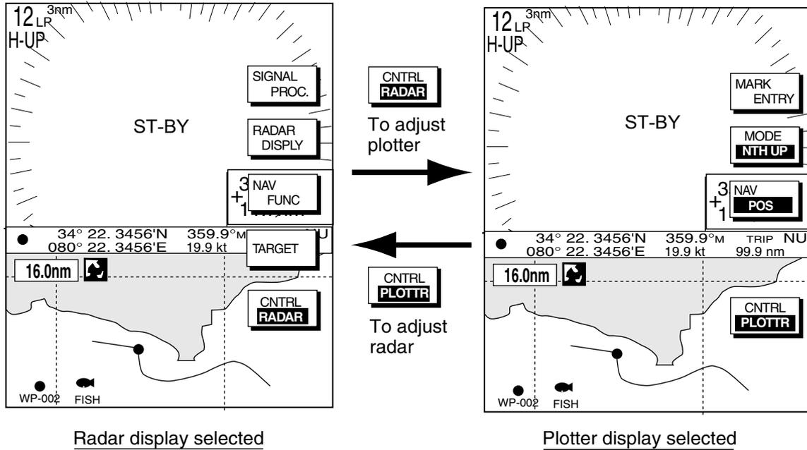
*How to switch control between modes in the plotter/sounder combination display*
