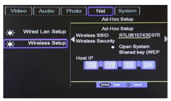
Save settings and test. After successful test, network information will be shown. Press ENTER to return to the Network Setup.
