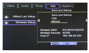
Set the name of product in wireless network as wireless SSID. Set the host IP address and make sure that the IP address does not conflict with the USB wireless network card IP addresses of your computer.
