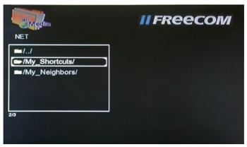
Press the "Option" button on the remote control. In the pop-up window select "add" to add a new shortcut. The user will be GUEST, as IP address the IP address of the computer in your peer-to-peer network has to be entered.
