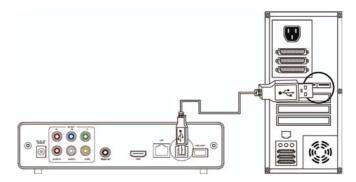
Follow the instructions as shown in the above picture and connect the device to PC. Power on the PC and enter the system. The PC detects the device automatically and then the device can be used as an external USB storage device. After data transfer is finished, please remove the USB storage device safely (click the USB device icon to stop the USB device and then pull out the USB cable).
