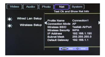
Press ENTER on the remote control. After the connection was established successfully, you will see a summary where IP address, subnet mask and default gateway are shown. Press ENTER again to return to the Network Setup. You will now see the IP address of your device and an indicator showing the signal strength of your connection.
