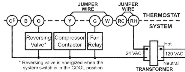
\* Reversing valve is energized when the system switch is in the COOL position
