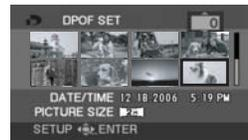
**3 Move the joystick up or down to select the number of prints, then press the joystick.**
