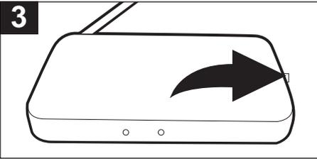
Slide the Receiver's POWER switch to the ON position; the red POWER indicator on the receiver will light. If the microphone is on, the green Microphone ON indicator on the receiver will also light. Raise the antenna for best reception and speak or sing into the microphone as desired.
