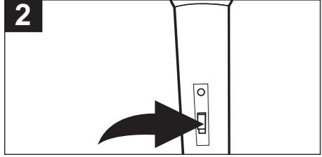
Slide the Microphone ON/STANDBY/OFF switch to the ON position; the POWER indicator on the microphone will light.
