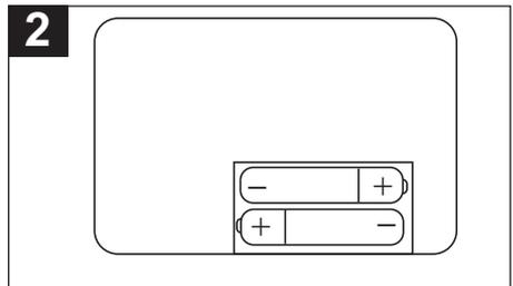
Insert two (2) "AA" size batteries (not included) following the polarity diagram (+/-). Slide the battery cover back into place.
