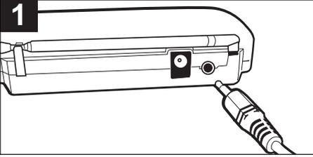
Insert the large end of the cord into the Microphone jack on the unit you are connecting this wireless microphone to, and the small end into the Line OUT jack on the receiver.
