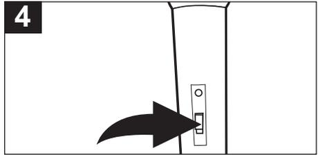
Slide the Microphone ON/STANDBY/OFF switch to the STANDBY (Standby) position to put the microphone in Standby mode (it will be on, but will not transmit). Slide the Microphone ON/STANDBY/OFF switch to the OFF position to turn the microphone off; the POWER indicator on the mic and the green MIC indicator on the receiver will go out.
