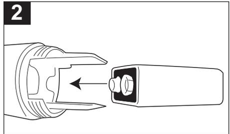
Insert one 9V battery, making sure to observe the correct polarity (+/-). Twist the battery cover clockwise to put it back on.
