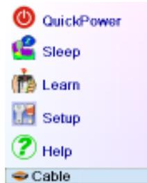
Only Devices you've previously set up are displayed. The others are grayed out. Press any key that isn't grayed out to send the "Power" command for that device.
