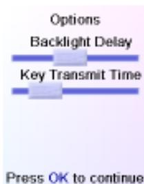
Key Transmit Time changes the delay between digits when sending favorites, e.g. 1-6-2. This can be used in situations where the channels are not accepted by the set-top box.
