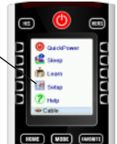
Press the **MODE** key, then select a device type to change the mode that the remote is in. E.G., if the remote is in Cable mode then the hard keys such as Channel Up/Down, Volume Up/Down, numbers, etc., operate your cable box.
