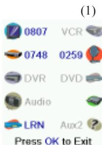
This screen also lets you view the codes for any device that's been set up. In the above example you can see the codes that are set for TV, Cable, and SAT. We've selected CD and can then enter its 4 digit code from the code list, using the number keys on the remote. The above also shows that we've learned codes under the AUX1 key in DVD mode.
