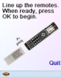
Next press the key (on the other remote) for the function you want to learn. Hold the key pressed until the screen says that the command was successfully learned. Note for some types of key you might need to hold the key pressed, but for other types a quick press is sufficient. Experiment a bit. If keys you learn are sent multiple times try learning them with just a quick press.
