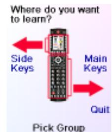
If you press a **right** Side Key (to select Main Keys) you are going to learn, say, the Chan Up key from an existing remote and store it under the Chan Up key on the IR10A remote. Or learn the Power key from an existing remote and store it under the Power key on the IR10A remote, etc.
