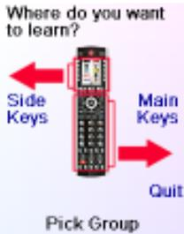
Select the device you want to learn keys for. In this example we only have a TV, Cable Box and Satellite Receiver set up, so the rest are grayed out, but you can still select any of the devices to learn commands for. E.G., in this case we selected DVR.
