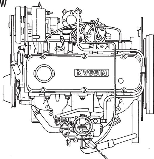
Figure 9. Nissan Model A15 Basic Engine Components
