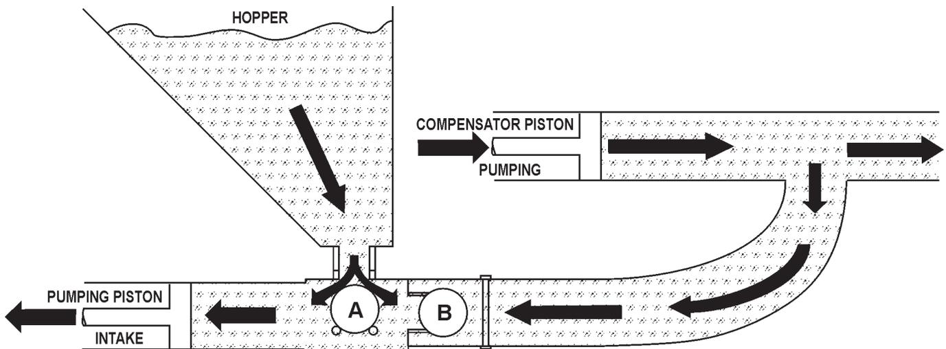
Figure 10. Pumping Cylinder
