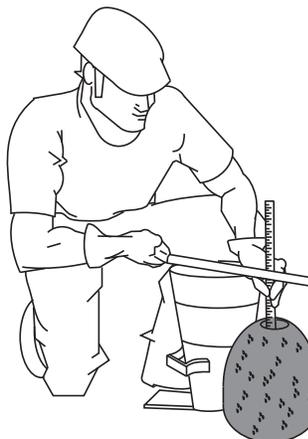
Figure 35-F. Slump Test (Measurement)
