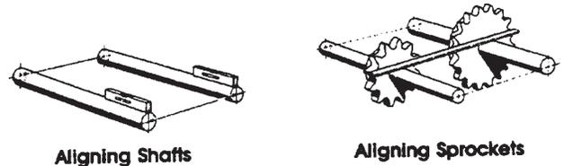
Figure 29. Shaft and Drive Sprocket Alignment
