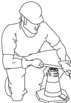
Figure 35-D. Slump Test (Removing Excess Concrete)
