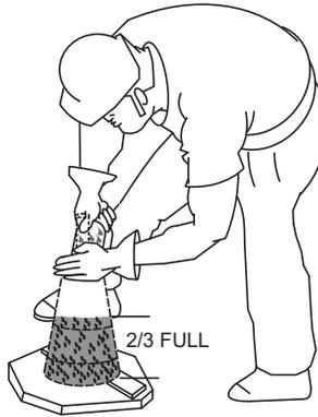
Figure 35-B. Slump Test (2/3 Full)
