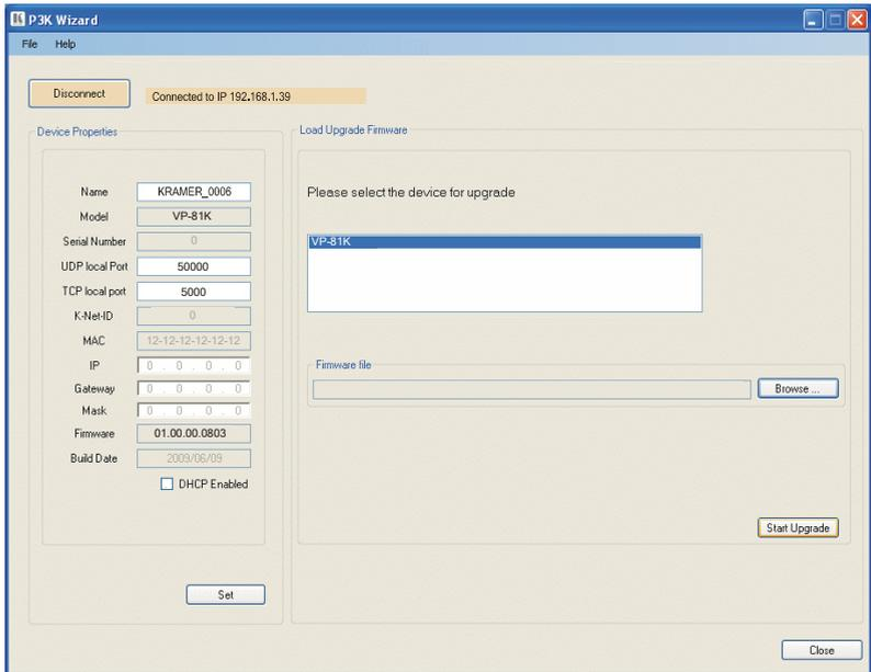
Figure 11: Device Properties Screen
