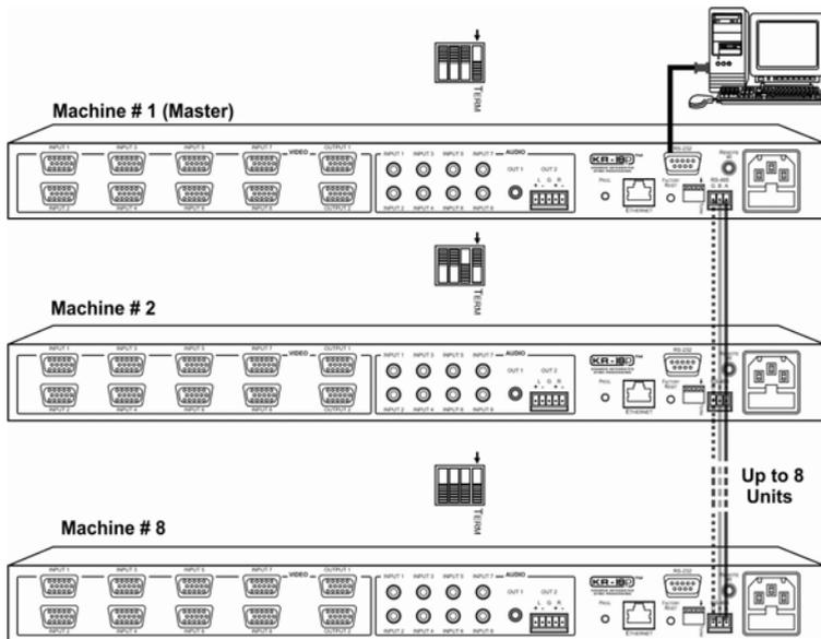
Figure 15: Control Configuration via RS-232 and RS-485
