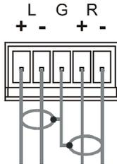
Figure 4: Connecting an Balanced Stereo Audio Output
