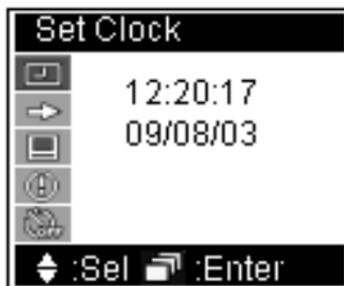
When setup is finished, push the switch until the setup screen disappears. Then the settings are successfully stored.
