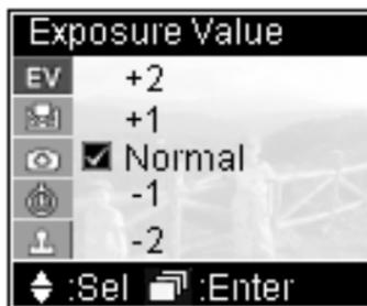
In addition to Normal, you can increase two levels up and decrease two levels down. Increasing Exposure Value will cause the image brighter whereas decreasing Exposure Value will get a darker image. You can make use the brightness change of the screen to gauge your adjustment.
