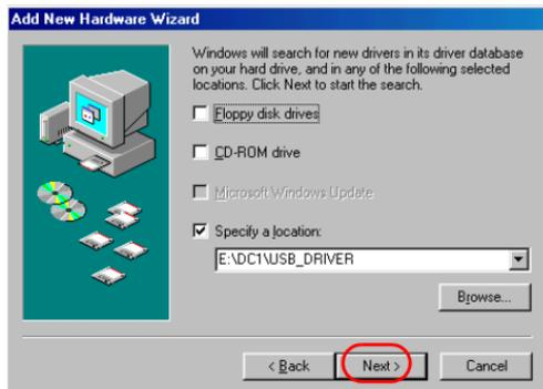
4. Windows® will find the SV2's USB driver in the companion CD. Click on the "Next" button to start installation. When completes, click on the "Finish" button to finish the driver installation.
