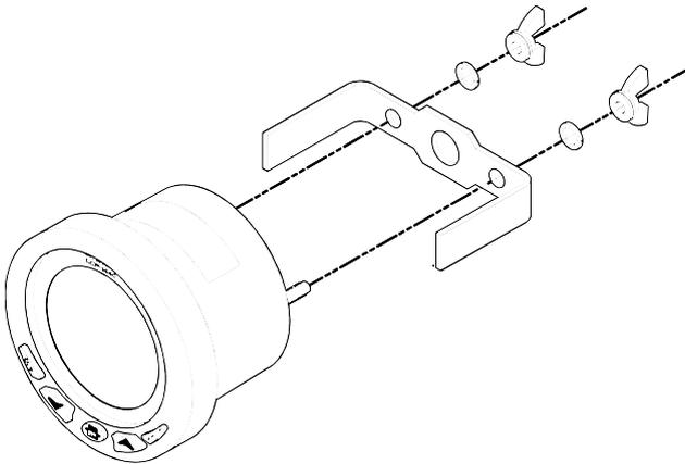
**Secure unit to the dash using "U" bracket as shown.**
