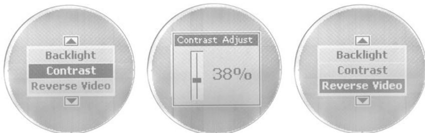
**Contrast is highlighted on the Screen menu (left). The Contrast Adjust window (center). Reverse Video highlighted on Screen menu (right).** The easiest way to change the look of the display is to utilize the Reverse Video command, commonly used for nighttime viewing.
