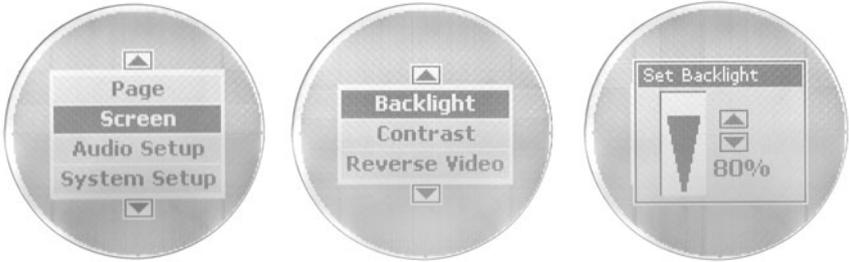
**Basic menu with Screen highlighted (left). Screen option menu (center) with Set Backlight window (right).**
