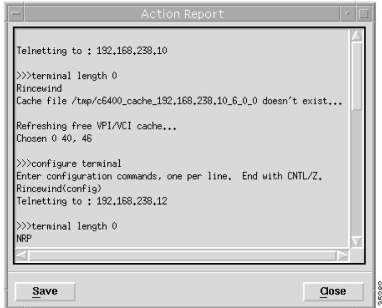
The Action Report window details the Cisco IOS commands executed when the service is commissioned. Invalid Cisco IOS commands result in a failure to commission the service.
