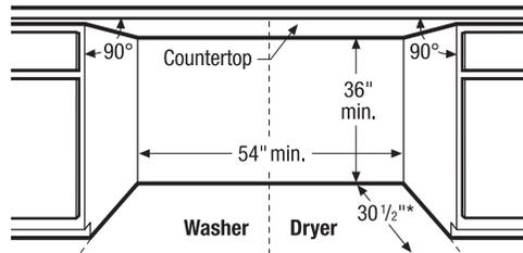
**Side-by-Side Units in Under-Counter Installation**
