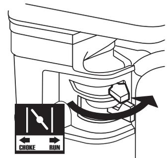
**NOTE:** Moving the Choke Lever too fast could stall the engine.
