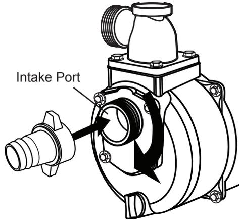
3. Slide one of the Hose Clamps over the end of the suction hose (a). Slide the Hose onto the Hose Coupler (b). Use a screwdriver (not included) to tighten the Hose Clamp until secure.
