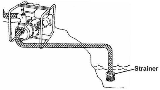
4. Secure the Intake Hose in place to keep it from moving once the Pump is turned on. The Intake Hose should be as short as possible for more efficient operation.
