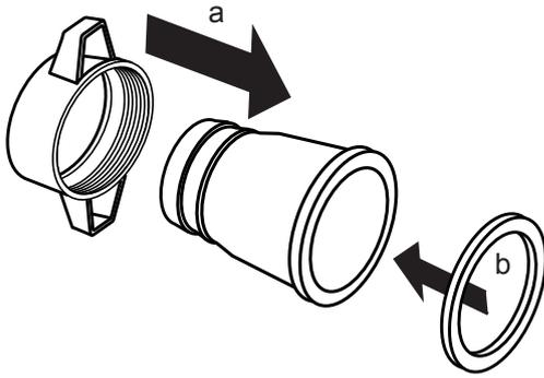
6. Thread the Hose Coupling Ring clockwise onto the Discharge Port until tightened securely.
