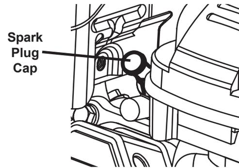
1. Disconnect spark plug cap from end of plug. Clean out debris from around spark plug.
