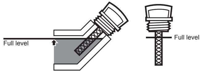
7. Add the appropriate type of oil until the oil level is at the full level. SAE 10W-30 oil is recommended for general use. The SAE Viscosity Grade chart shows other viscosities to use in different average temperatures.
