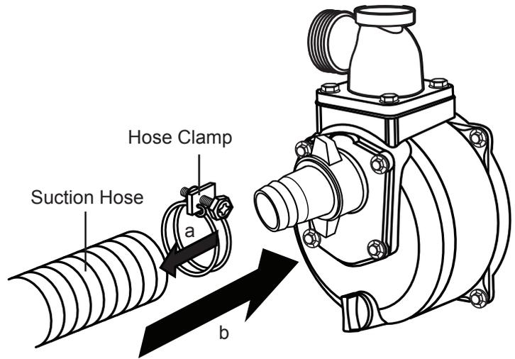
4. Slide a Hose Clamp over the other end of the suction hose (a). Slide the Intake Strainer into the end of the suction hose (b). Use a screwdriver to tighten the Hose Clamp until secure.
