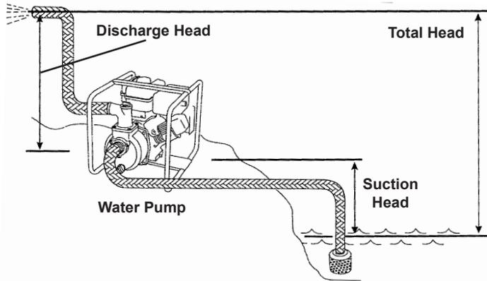
As the head (pumping height) increases, pump output decreases. The length, type, and size of the suction and discharge hoses can also significantly affect Pump output.
