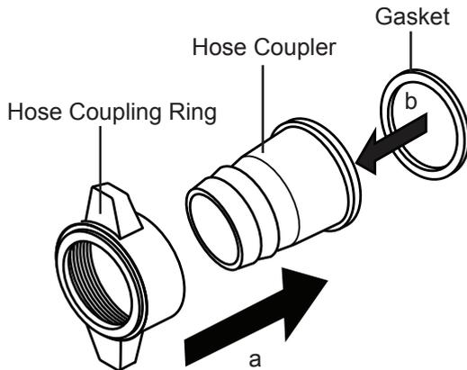
2. Thread the Hose Coupling Ring onto the Intake Port (a), and turn clockwise until fastened securely (b).
