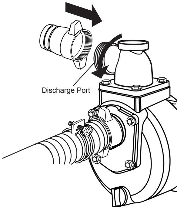
7. Slide a Hose Clamp over the end of the Discharge Hose (a). Slide the Discharge Hose onto the Hose Coupler (b). Use a screwdriver to tighten the Hose Clamp until secure.
