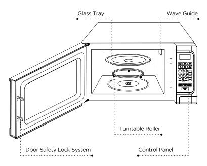
NOTE: Do not remove the mica plate covering the wave guide in the oven cavity.
