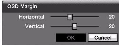
Use the horizontal and vertical sliders to adjust the horizontal and vertical margins so that text and icons are not hidden beyond the edges of the monitor.
