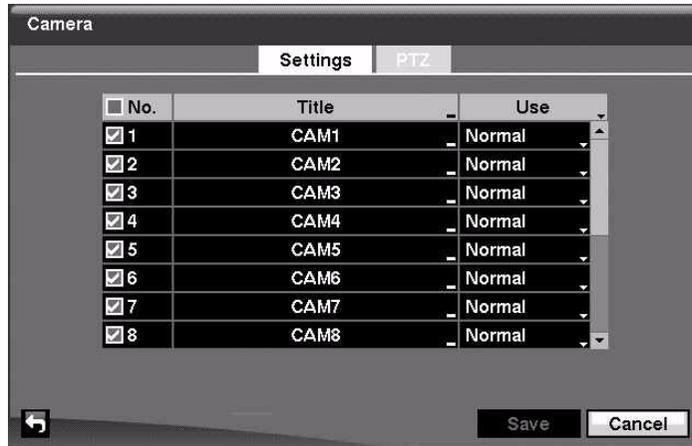
To turn the camera number **On** or **Off**, select the field under **No.** and press  $\left(\frac{F}{N}\right)$ .
