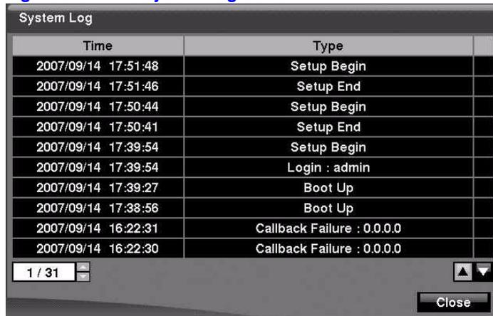
2. Select log entries by either scrolling through the log pages by using the **UP** and **DOWN** arrows, or by choosing a log page directly by entering the log page number in the field at the bottom left of the screen.
