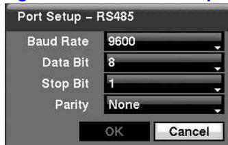
3. Use the ATM or POS manufacturer's recommended settings when configuring the RS-232C, RS485 or USB-Serial ports. You need to know the Baud Rate, Data Bit number, Stop Bit number, and Parity. Highlight **OK** and press  $\left(\frac{1}{2}\right)$  to load the settings.
