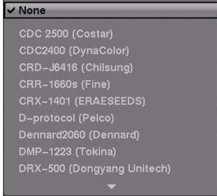
3. Select your camera from the list and press **(F10)**. You need to connect the camera to the RS-232C or RS485 connector on the back of the DVR following the camera manufacturer's instructions.
