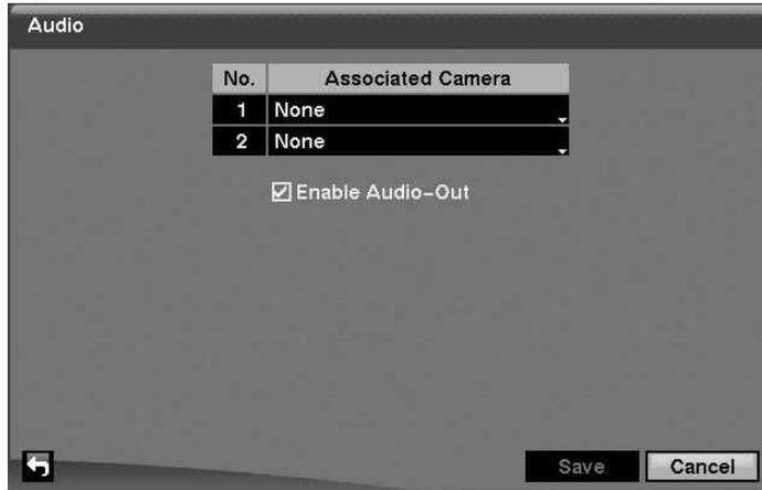
2. Highlight the field beside the input and press **(F11)**. A list of cameras appears, and you can select which camera you want associated with that audio input.
