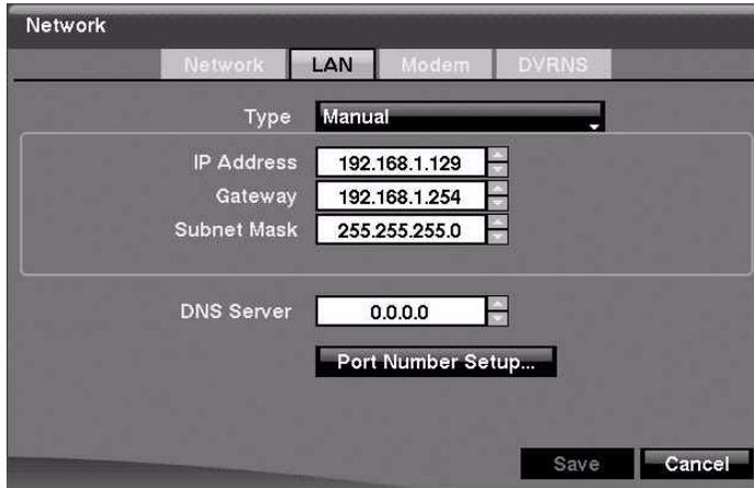
2. Highlight the field beside **Type** and press  $\uparrow/\downarrow$ . You can select the type of network configuration from: **Manual**, **DHCP**, and **ADSL (with PPPoE)**.
