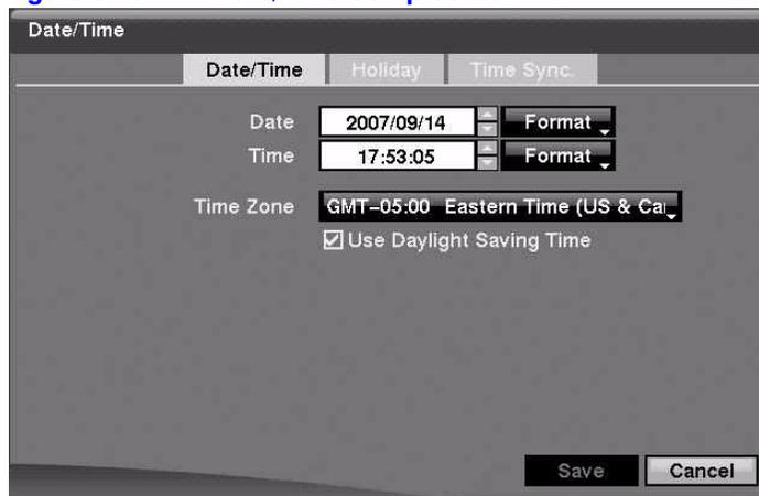
2. Highlight the first field beside **Date** and press **↵**. The individual sections of the date highlight. Use the **UP** and **DOWN** arrows to change the number. Use the **LEFT** and **RIGHT** arrows to move between month, date, and year. Press **↵** when you have the correct date.
