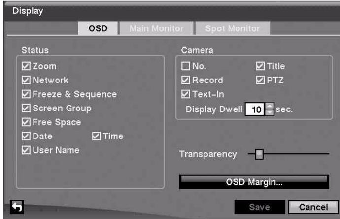
To toggle an item **On** and **Off**, highlight it and press . When an item is **On**, there is a checkmark in the box beside it. The following items can be turned **On** or **Off**:
