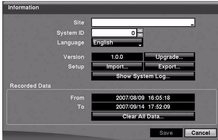
2. Highlight the **Site** field in the Information screen and press  $\left(\frac{\text{v}}{\text{n}}\right)$ . A virtual keyboard appears that you can use to enter a Site Name.
