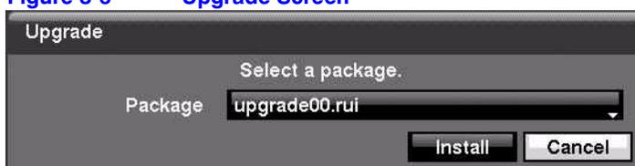
The screen displays the upgrade package file names that are available. The .rui extension indicates that the file is for software upgrades.
