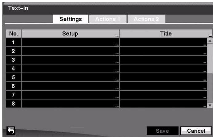
Highlight the field under the **Setup** heading, and press **F4**. Selecting the **Setup** heading changes all the parameters, excluding Port settings, of all the text input channels.
