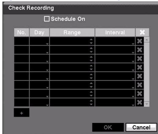
2. Highlight **Schedule On** and press  $\left(\frac{1}{n}\right)$  to toggle the schedule **On** and **Off**. When set to **On**, the rest of the Check Recording screen becomes active.
