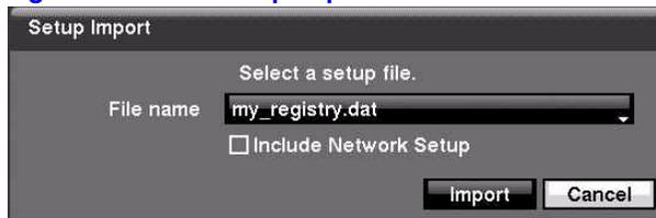
3. Select the desired setup file and press **Import** to import the selected settings and change the DVR settings accordingly.
