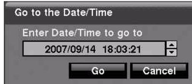
2. Move the cursor over the date and time and then press  $\odot/\square$  (Play/Pause). Use the Left and Right arrow buttons to highlight the year, month, day, hours, minutes and seconds. Use the Up and Down arrow buttons to change to the date and time for which you want to search for video.
