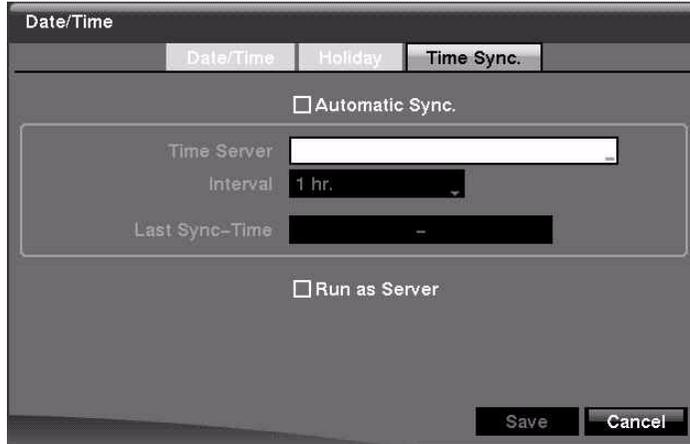
2. Highlight the field beside **Automatic Sync.** and press  $\left(\frac{\text{v}}{\text{u}}\right)$  to toggle between **On** and **Off**. When set to **On**, the Time Server and Interval fields become active.
