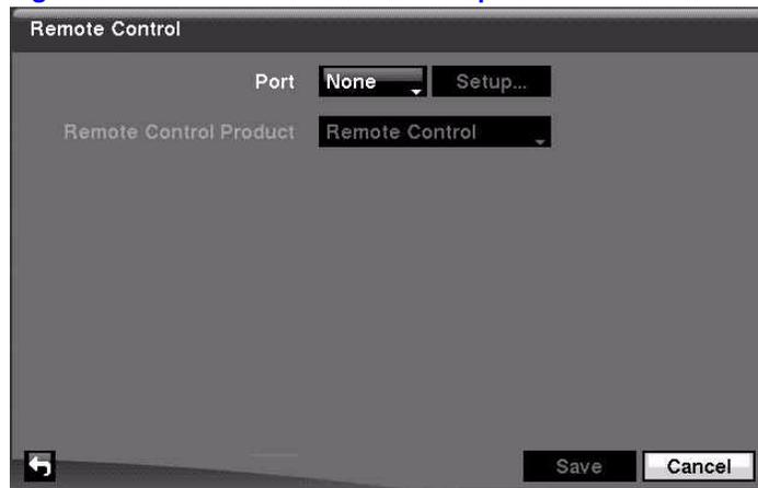
2. Highlight the field beside **Port** and select from **None**, **RS-232C**, and **RS485**. If the RS-232C port and RS485 port are in use for PTZ control, networking, or text input, the remote keyboard cannot be configured.
