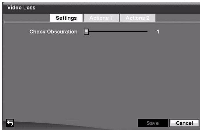
2. Highlight the slider bar beside **Check Obscuration**, and use the **LEFT** and **RIGHT** arrows to adjust the setting. The sensitivity can be set from **Never** to **15** (extremely sensitive).
