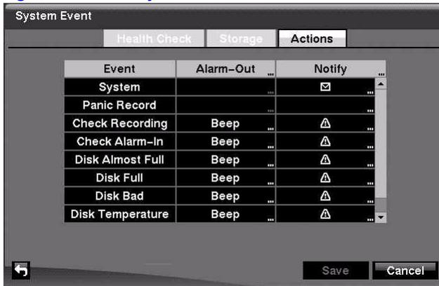
2. Highlight the **Alarm-Out** field beside the desired event (Check Recording, Check Alarm-In, Disk Almost Full, Disk Full, Disk Bad, Disk Temperature, or Disk S.M.A.R.T.), and press **F7**. A list of Alarm Outputs appears.
