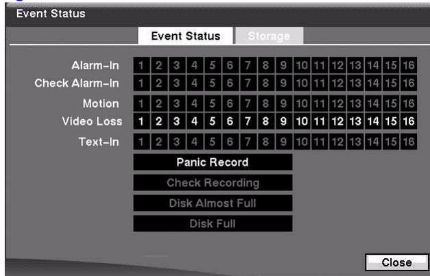
**Alarm-In**, **Motion**, **Video Loss** and **Text-In** highlight when each event is detected based on the settings you made in the Alarm-In, Motion Detection and Text-In setup screens on the Event menu.
