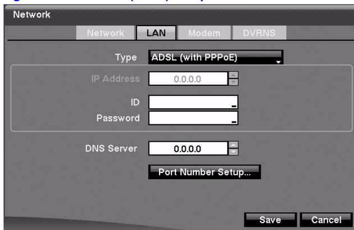
2. Highlight the field beside **ID** and press  $\text{F}_7$ . A virtual keyboard appears so you can enter the ID for ADSL connection.
