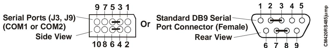
Figure 3-1. Serial 1 to RS485 Conversion
