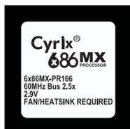
6x86MX-PR166      60MHz Bus 2.5x      2.9V (or as marked)
