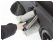
The filter and brushes can be accessed quickly and easily without tools for service and replacement.
