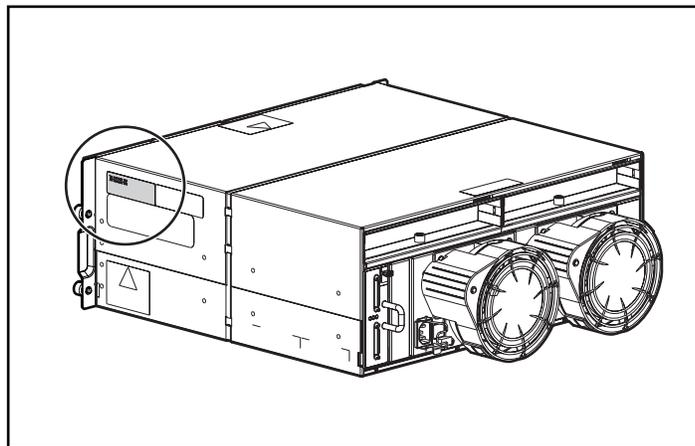
12. Install all the removed components in the new chassis. To replace each component, refer to the procedures in this chapter.
