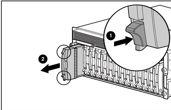
To replace a blank, slide the blank into the bay until it locks into place.
