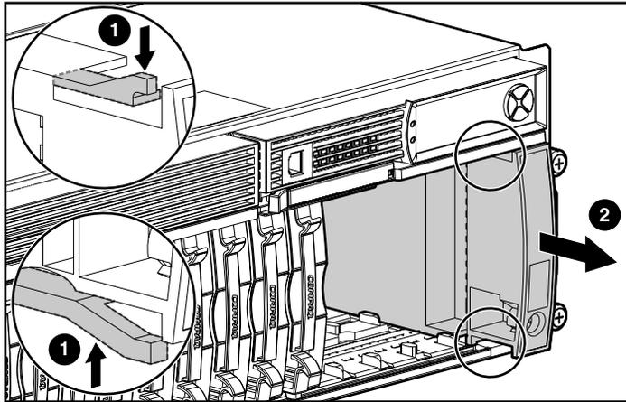
To replace the component, slide the power button/LED assembly into the bay until it locks into place.
