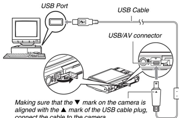
*Making sure that the ▼ mark on the camera is aligned with the ▲ mark of the USB cable plug, connect the cable to the camera.*
