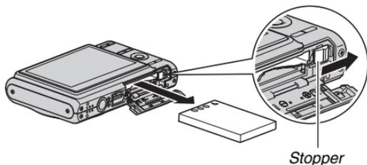
3. While still holding the stopper, pull the battery out the rest of the way.
