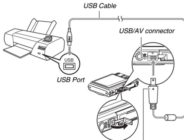
*Making sure that the ▼ mark on the camera is aligned with the ▲ mark of the USB cable plug, connect the cable to the camera.*
