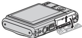
While pressing lightly on the cover, slide it in the direction indicated by the arrow to open.
