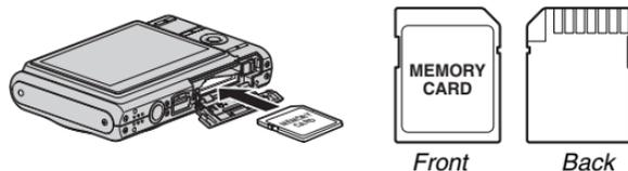
With the front of the memory card facing upwards (towards the monitor screen side of the camera), slide it into the card slot and press until it clicks securely into place.
