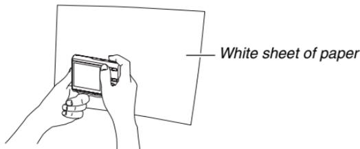
The camera will adjust white balance settings for the current conditions, and display "Complete" when it is finished.
