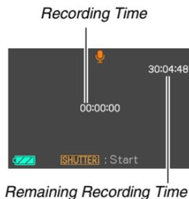
**3. Press the shutter button to start recording.**
