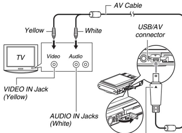
Making sure that the ▼ mark on the camera is aligned with the ▲ mark of the AV cable plug, connect the cable to the camera.
