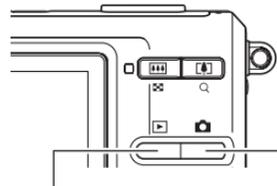
To view images, press [▶] To record, press [📷] to power up in the PLAY mode. To power up in the REC mode.
