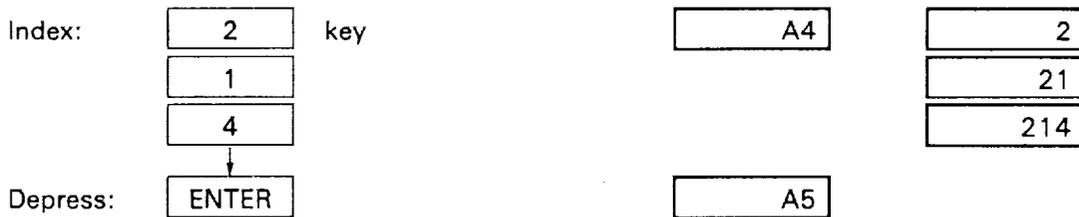
**NOTE:** As with time setting routine the SL59 will check details of input, if number entered is over 255 then SL59 will error.
