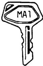
This key (MA1) will access the PR2, PR1, REG, OFF and X positions.
