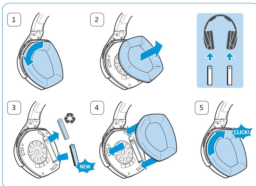
**i** You can also power the headphones using standard batteries (AAA size, 1.5 V). Note however, that standard batteries are not rechargeable, and if you are using non-rechargeable batteries, you must not place the headphones on the headphones holder.
