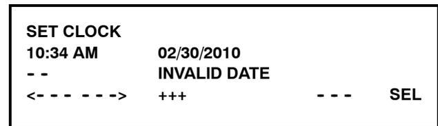
When the MENU/SEL key is pressed, the controller will return to the previous LCD screen to allow for correction of the calendar entry. The controller will not advance to the next screen until a valid date has been entered. Once a valid date has been entered, pressing the MENU/SEL key will display a the Daylight Saving Time screen.
