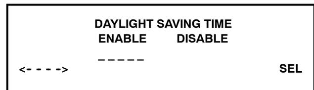
Pressing the <- - arrow key or the - -> arrow key will move the cursor left or right respectively. Pressing
