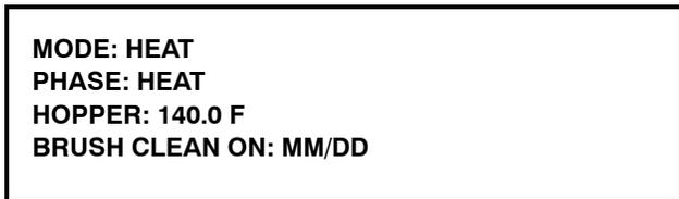
During the heating phase, the mix temperature must be raised above 151°F (66.1°C) within 90 minutes or the freezer will be locked in STANDBY, and the cycle failure display will appear.
