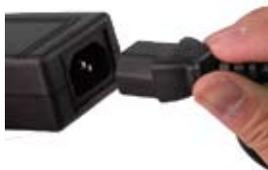
3. Plug the 4 pin power adapter to your ATA/ATAPI device
