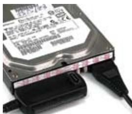
4. Plug the power adapter to power source and turn on the power .
