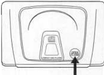
4. Place a CD/CD+G in the compartment tray over the center hub, label side up.
