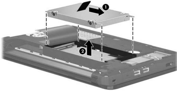
Reverse this procedure to reassemble and install the hard drive.
