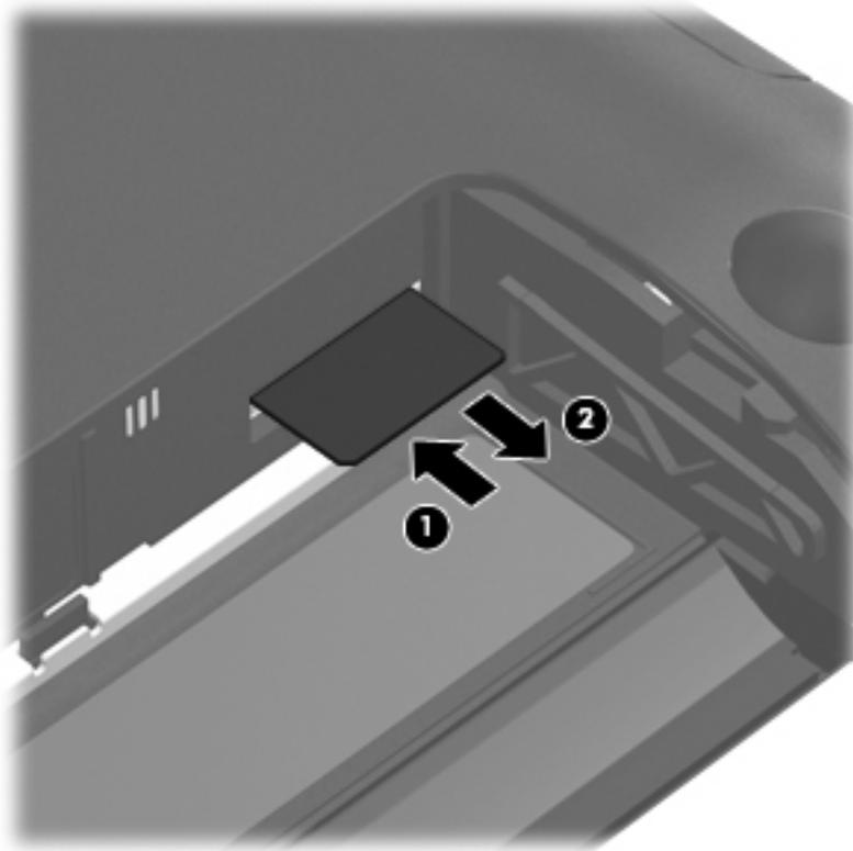
Install the SIM by inserting it into the SIM slot until you hear a click.
