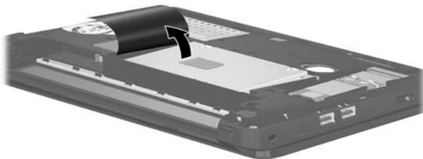
2. Using a small Phillips screwdriver, remove the 4 hard drive mounting screws.
