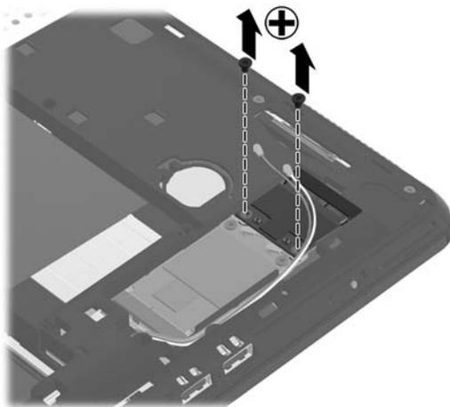
3. Lift up and remove the WLAN module at an angle.
