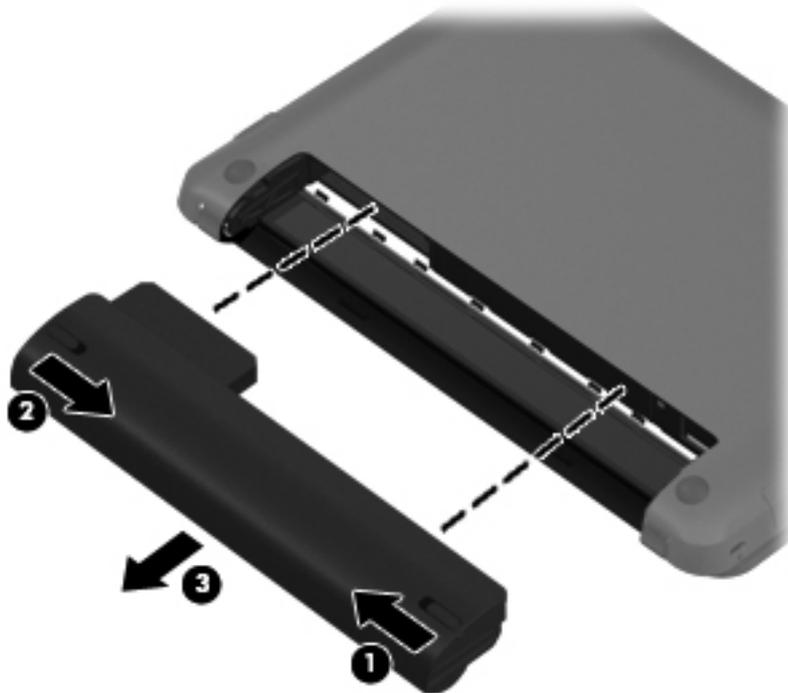
Reverse this procedure to install a battery.
