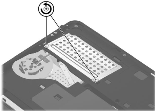
2. Lift up and remove the memory shield.
