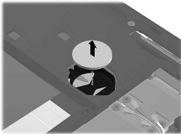
Reverse this procedure to install the RTC battery. When installing the RTC battery, make sure the “+” sign faces up.
