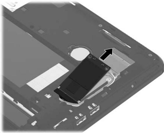
Reverse this procedure to install the WWAN module.
