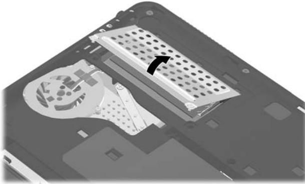
3. Using your fingers, spread the 2 retention clips outward until the memory module tilts up at a 45-degree angle.
