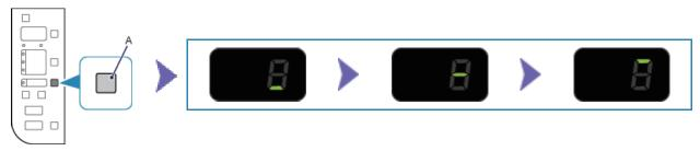
2. Make sure that the LED flashes as shown in the illustration above, then press and hold the WPS button on the access point within 2 minutes.
