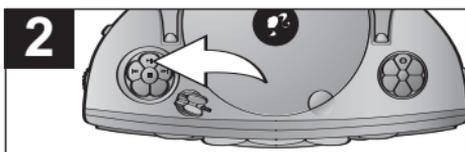
Slide the **FUNCTION** switch to the **CD** position to turn the unit on and select **CD** mode; the **POWER** indicator will light.
