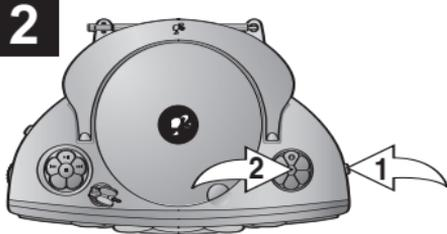
Slide the BAND switch ❶ to select AM, FM or FM ST. (Stereo). Tune a desired station by turning the TUNING control ❷.
