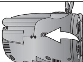
To turn the radio off, slide the FUNCTION switch to the OFF position; the POWER indicator will turn off.
