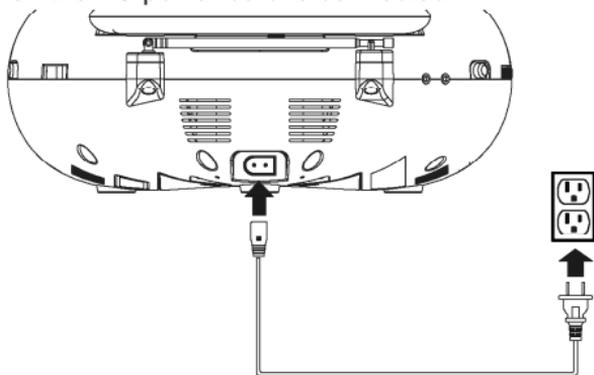
**NOTE:** The AC plug supplied with the unit is polarized to help minimize the possibility of electric shock. If the AC plug does not fit into a nonpolarized AC outlet, do not file or cut the wide blade. It is the user's responsibility to have an electrician replace the obsolete outlet.
