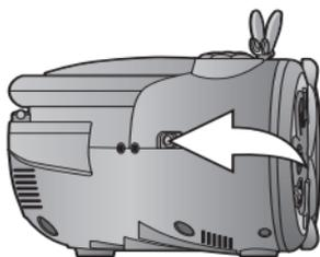
Slide the FUNCTION switch to the RADIO position to turn the unit on and select Radio mode; the POWER indicator will light.
