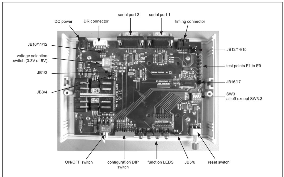
Figure 3-5 Internal layout of the development unit
