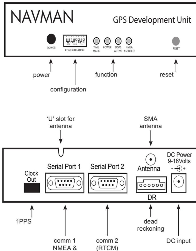
**Figure 3-1 Front and back panels of the Jupiter 30 development unit
