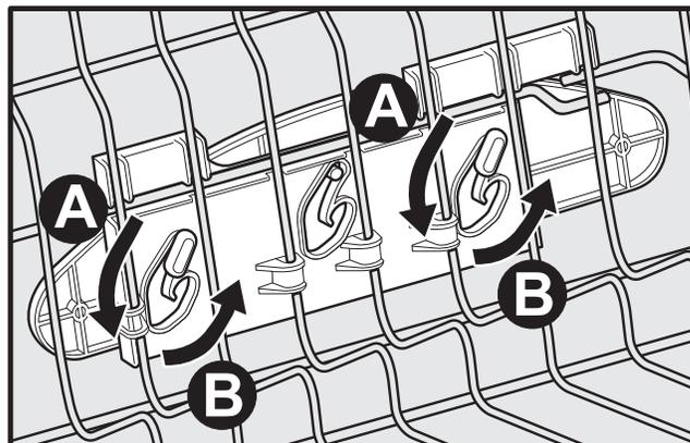
To lower the upper rack, lift the rack straight upward and push rack slightly towards the rear of the dishwasher as it is lowered.
