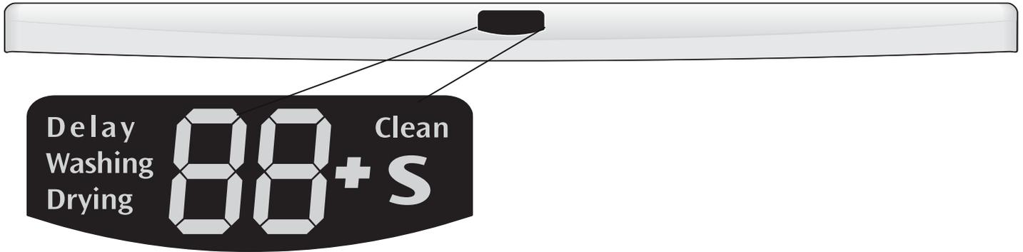
The WASHING light comes on at the beginning of cycle and remains on until the end of the main wash.
