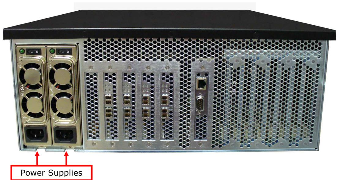
**Figure 29 - Back of RamSan-500, Power Supply Location**
