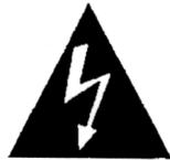
The lightning flash with arrowhead within a triangle is intended to tell the user that parts inside the product are a risk of electric shock to persons.
