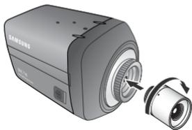
3. Set focus of camera using Back Focus Control Lever of camera side after combining C-Mount lens.
