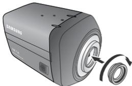
2. Turn the C-Mount lens clockwise to install it.
