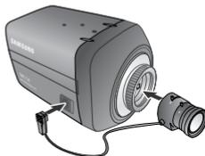
5. Set focus of camera using Back Focus Control Lever of camera side after combining Auto Iris lens.
