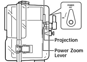
⚠ If the camcorder's Power Switch is not set properly when the camcorder is placed in the marine case, it could break and/or it could damage the Power Lever aligning boss on the marine case.
