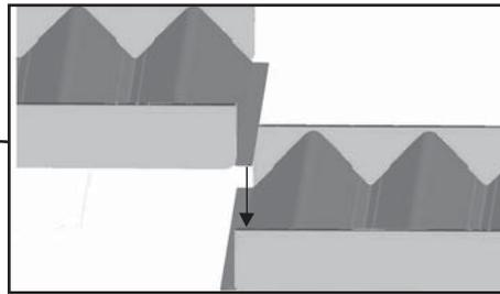
**IMPORTANT:** Stainless steel emitters must be placed keeping both flat walls overlapped to prevent any flare-up.
