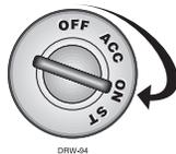
To disarm the security system, turn the ignition key on and press the Valet® switch the preset number of times within 15 seconds. If the system does not disarm, you may have waited too long; turn the ignition off and repeat the process.
