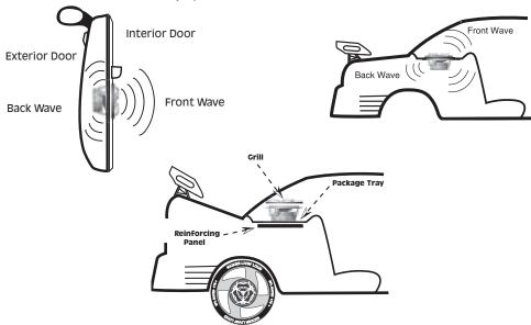
The ideal mounting scheme is to have a sturdy panel to cut out or to reinforce an existing panel with Masonite or medium density fiberboard. If the panel can flex at all, it will decrease the output of the driver and keep it from sounding it's best.
