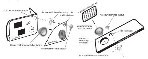
If custom mounting locations are desired for your drivers, check for interference from other mechanical systems in the vehicle. Watch for window mechanisms, hinges, trunk springs, wire harnesses, and anything that would be affected by the installation of these drivers. If metal must be cut to mount the speakers, try to avoid structural metal and braces. Once a location is chosen, cut the appropriate sized holes for the drivers.
