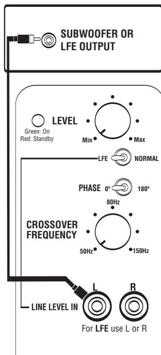
If your receiver/processor does not contain a Dolby Digital or DTS processor but has subwoofer outputs:
