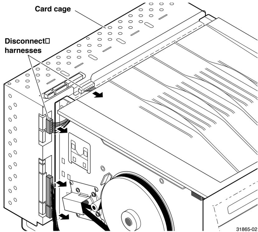
9. Lift out the engine control board.
