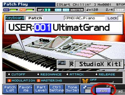
You can select patches on the Patch Play screen by highlighting the patch number—as shown above—or bank name, and then turning the VALUE dial. (We'll explain banks in a few pages).
