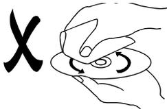
Do not wipe in a circular direction (Concentric scratches in the disc groove tend to cause noise.)
