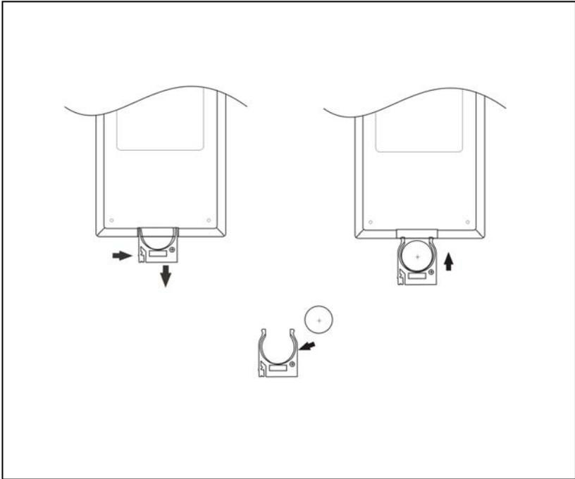
1. Referring to the drawing above, remove the empty battery receptacle.
