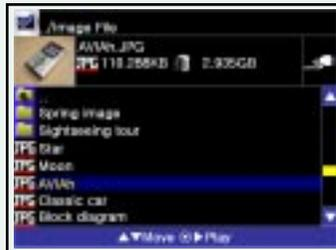
After moving to a desired file, pressing the **OK** Button will allow you to preview in a small screen in the upper left side.
