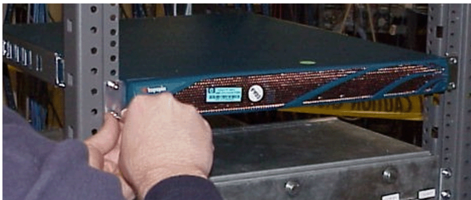
Figure 1-6: Secure Switch with Screws through the Front of the Rack
