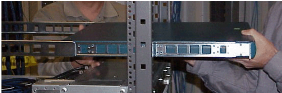
Figure 1-5: Sliding the Switch Into the Rack
