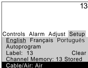
Press MOVE ◀ or ▶ to select Cable or Air. Select Cable if you have cable. Select Air if you have a home antenna connected to your TV.
