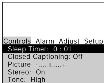
When 0:01 appears on the screen, the TV will shut off in one minute. Press VOLUME + to add more time.
