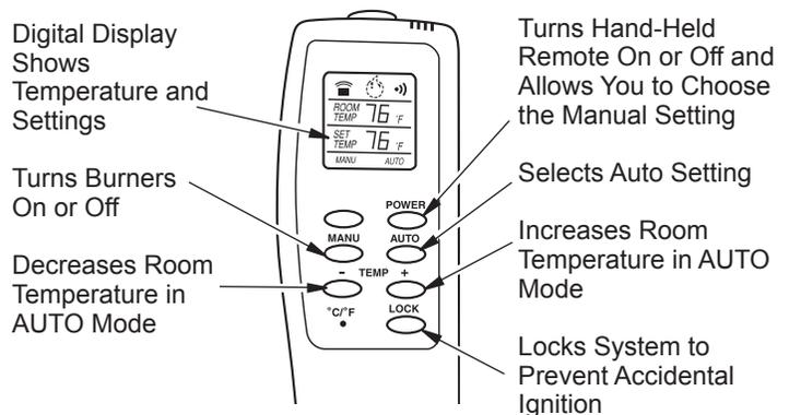
Figure 48 - Thermostat Hand-Held Remote Control Unit GHRCTB
