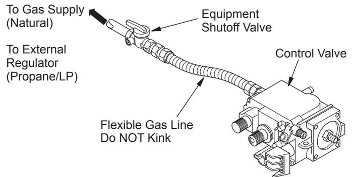
**Figure 32 - Connecting Flexible Gas Line to Millivolt Valve**
