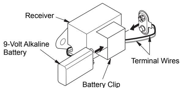
**Figure 37 - Attaching Alkaline Battery to Receiver**
