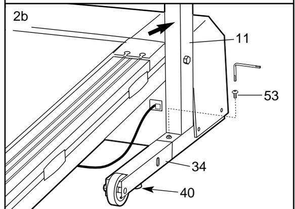
Attach the Extension Leg (34) with an Extension Leg Screw (53). Note: If there are short and long Extension Leg Screws, use the **long** Screw. **Make sure to push on the head of the Screw while tightening it.**
