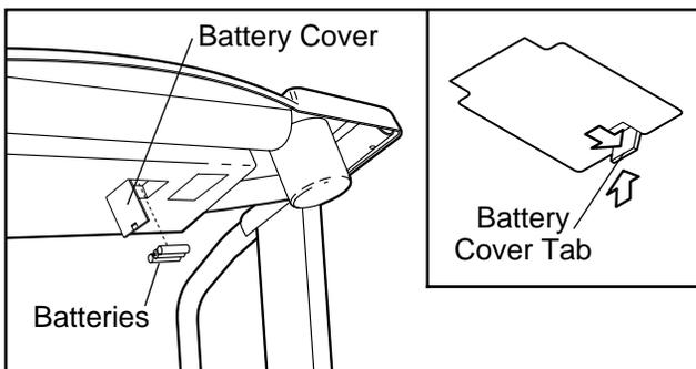
springs. Close the battery cover, push up on the tab, and then push the tab forward as shown. Be sure that the tab locks into place.
